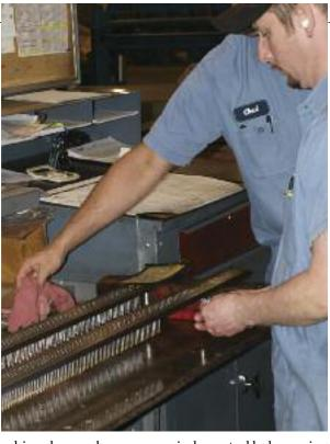
the perforated part, we can precisely control hole spacing. The web typically should be equal to or larger than the material thickness."
